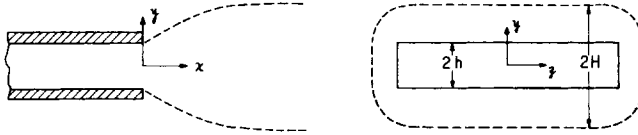
Fig. 3. Die swell from a slit die.
